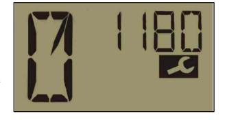
To leave the diagnostic mode, either shift the machine out of neutral or turn the keyswitch off and on. **NOTE:** Any movement of the tires will also take the machine out of the diagnostic mode.
